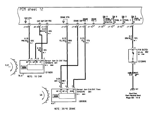
Figure 3.2.1a - XIII - P/Truck - Mechanization Diagram - Engine Crank & Cam Sensors
